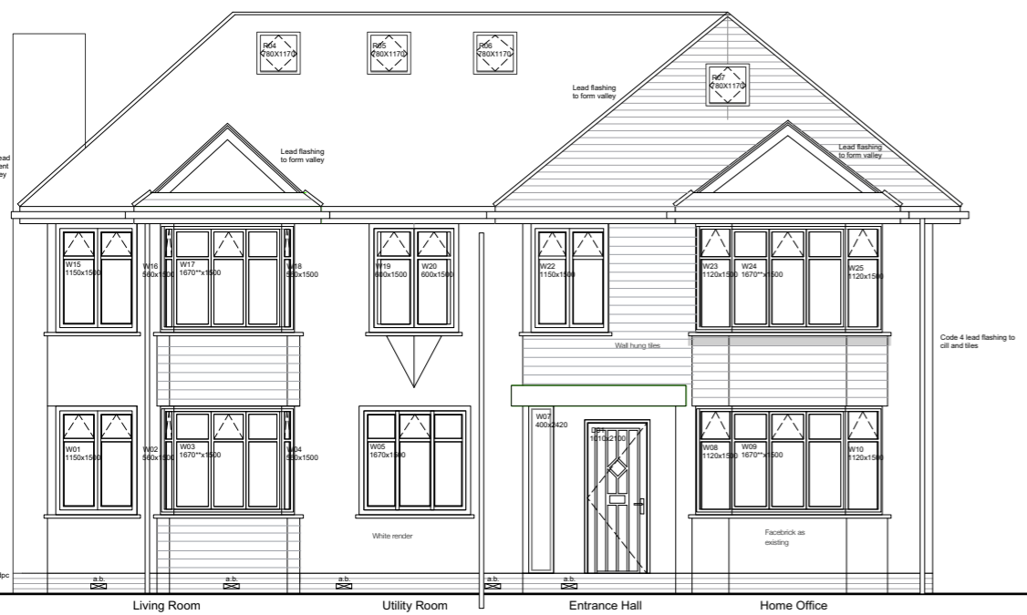
East Elevation [Front] 1:50
